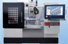
**EM69P** 5 Axis CNC Multi Purpose Machining center with Automatic Tool Changer
