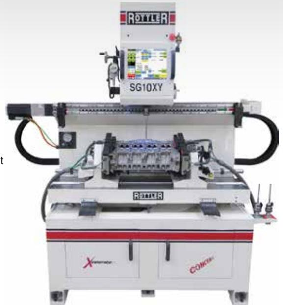
valve seat cutting such as valve seat housing counterboring and valve guide reaming, the spindle is required to be locked vertically. The ACTIV spindle has a pneumatic locking system that locks the spindle sphere rigidly vertically for other types of machining requirements.
