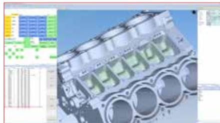
The advanced software design allows professional engine builders and head developers to maximize production and minimize preparation time. The next generation CNC control gives even greater capability beyond porting by letting users probe parts for duplication and modification all within the machine control – no external or third-party software or equipment required.
