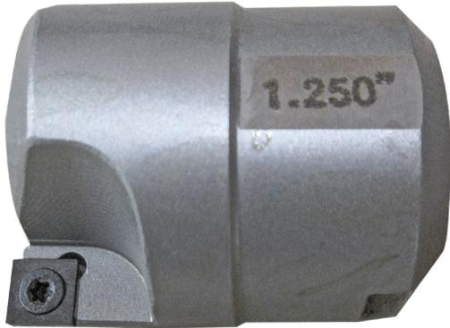
**FMH13125R1 1.3125" Fixed Double Replaceable Insert Milling Head**
