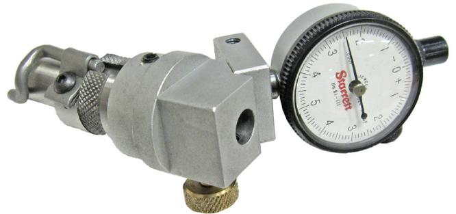
**VSG102-6MM Precision Valve Seat Concentricity Gage Base**
