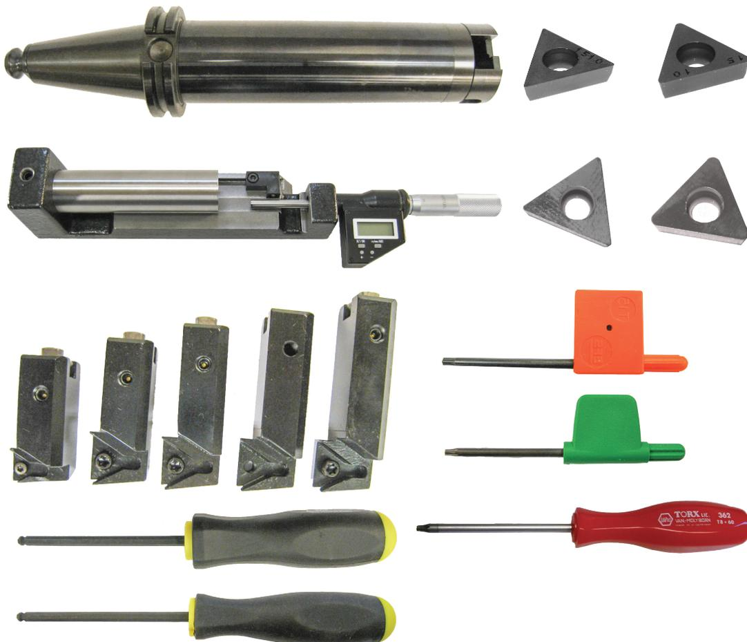
**Tool Holders for Brazed Tool bits (Chamfering) on Cutterhead 650-2-1D**
