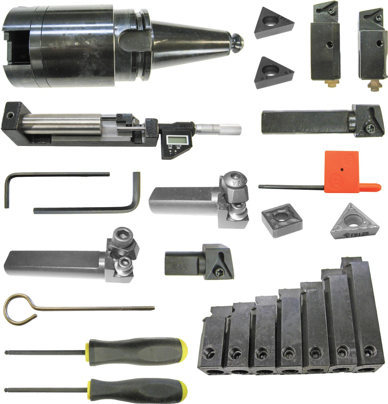
**RTCR322 Insert, Triangular Positive Rake, 3/8 IC 1/64" (9.397mm) Radius**
