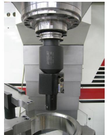
Special double diameter cutterheads allow both big end and small end to be bored in one automatic cycle. These cutterheads have pre-settable cartridges and can be adjusted in .0002" (.005mm).
