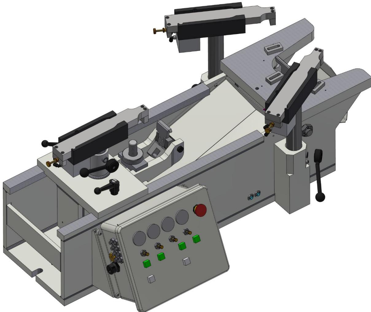
**690-3-70 Automatic 4Th Axis Block Roll Over Fixture**
