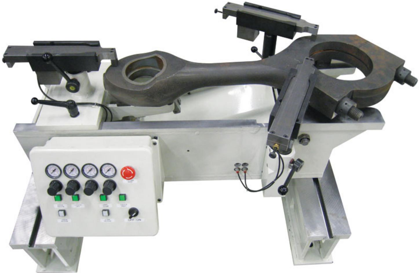
**650-3-66 Rottler Precision Compressor Conrod Cap Surfacing Fixture**
