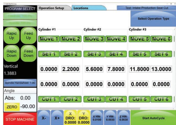
Multiple Cylinders/Valve Guides are programmed so that the SG100XY can move automatically from guide-to-guide – unattended. The slider allows 24 valve guide centers to be programmed in X and Y location.
