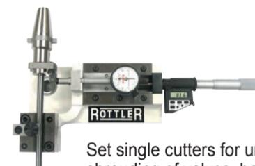
Set single cutters for unshrouding of valves, bowl work or seat ring removal.
