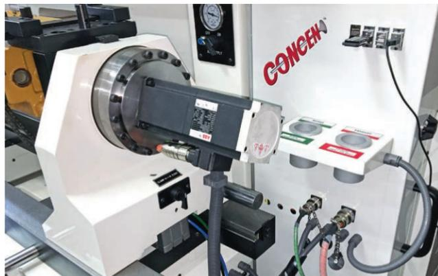
Rottler fixtures are designed to be changed easily and fast. Connections are screw type for quick disconnect.
