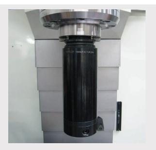
Rottler Boring and Sleeving Cutterhead installed in massive heavy duty EM69P Spindle.
