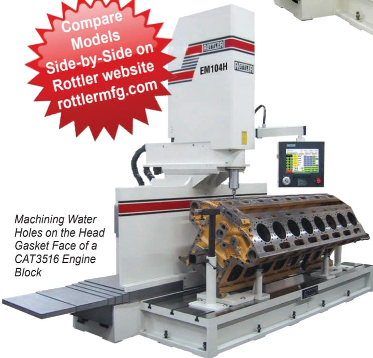
Machining Water Holes on the Head Gasket Face of a CAT3516 Engine Block
