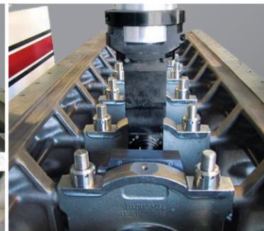
Special steel main bearing housings found in high power diesel engines such as MTU 4000 require high speed machining to obtain superior accuracy of roundness, straightness, parallelism and surface finish.
