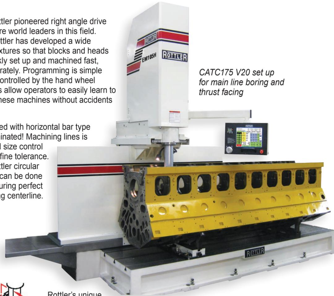
CATC175 V20 set up for main line boring and thrust facing
