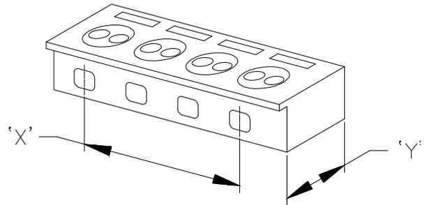
Position rear support blocks and front support blocks to hold the head approximately centered on the table top and spaced apart per dimensions measured in step '1' above. Generally, place the front blocks closer together than the rear blocks. If necessary, use either 2 or 4 spacers to raise the head for clearing studs or to angle the head so the cutterhead clears the head clamp handle assembly.
