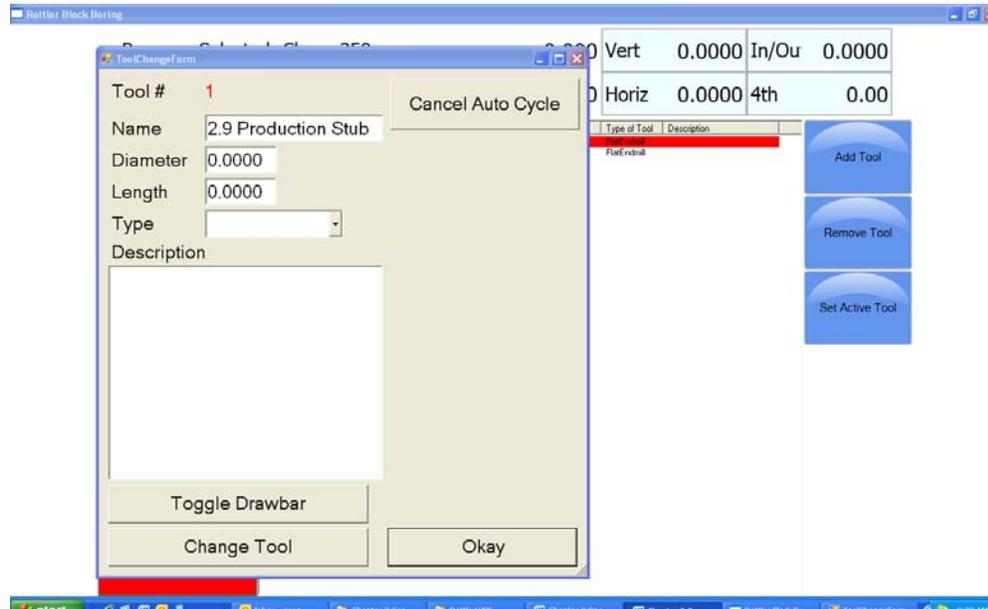
This window will open when the machine does an automatic tool change. This will be discussed in Chapter 3 Operating Instructions. After you press OK another window will open. This is a Warning Dialog box to inform the operator of the possibility of the spindle start if the tool change is done in an automatic program. Press OK.
