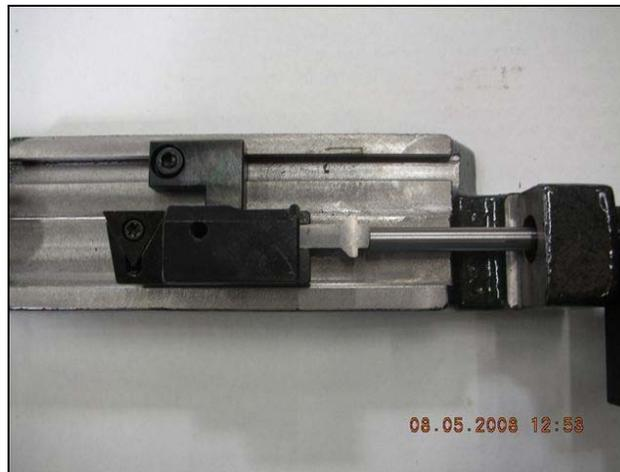
Slide the large diameter anvil up until it touches the end of the cutting tip of the tool holder. Tighten the set screw.
