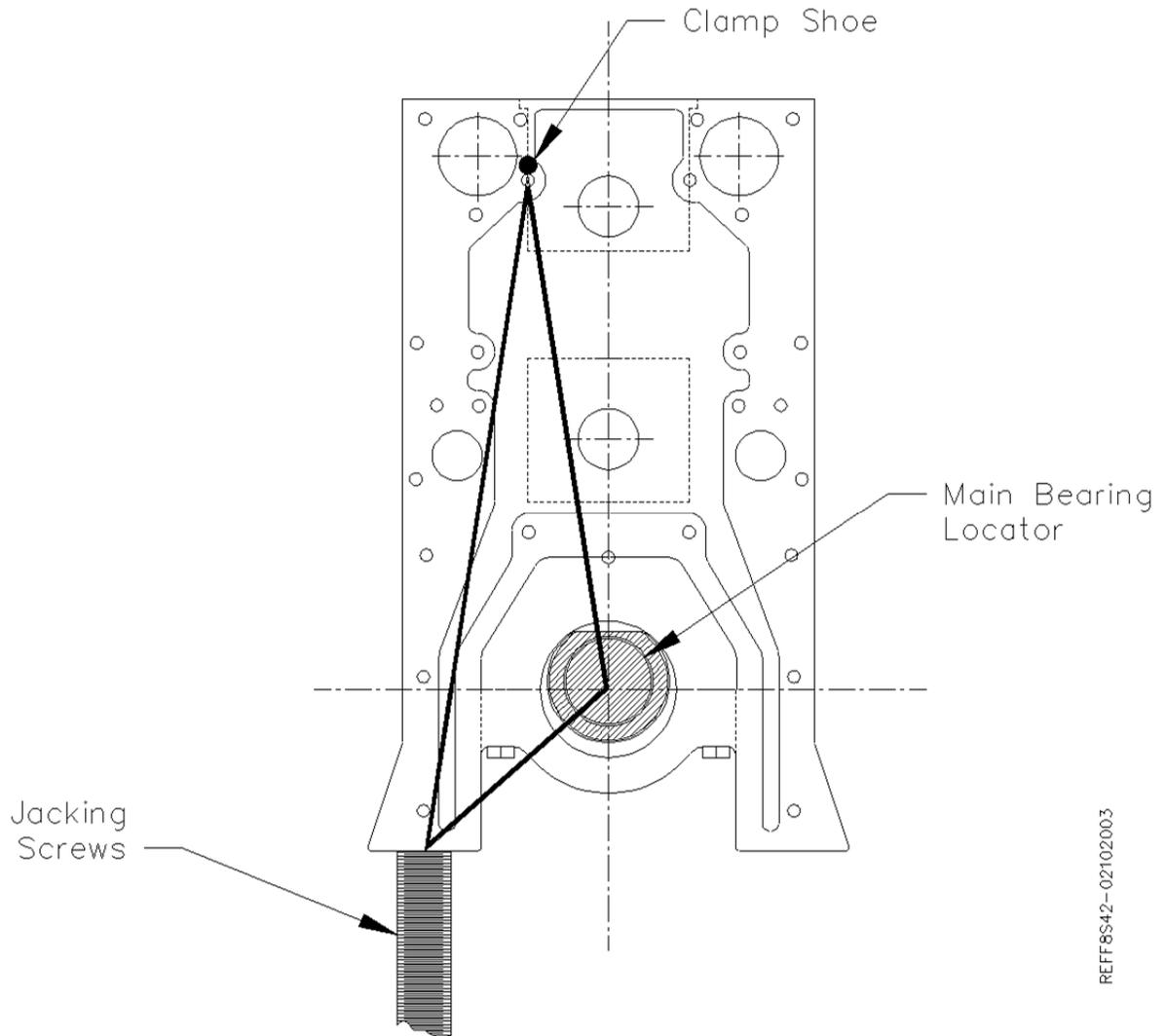
Adjust the height so the shoes rest on the clamp points. Tighten the clamp leg handles. Actuate the clamp shoes by turning their knobs. Apply pressure to the two clamps as evenly as possible to avoid tipping the block up on one side.
