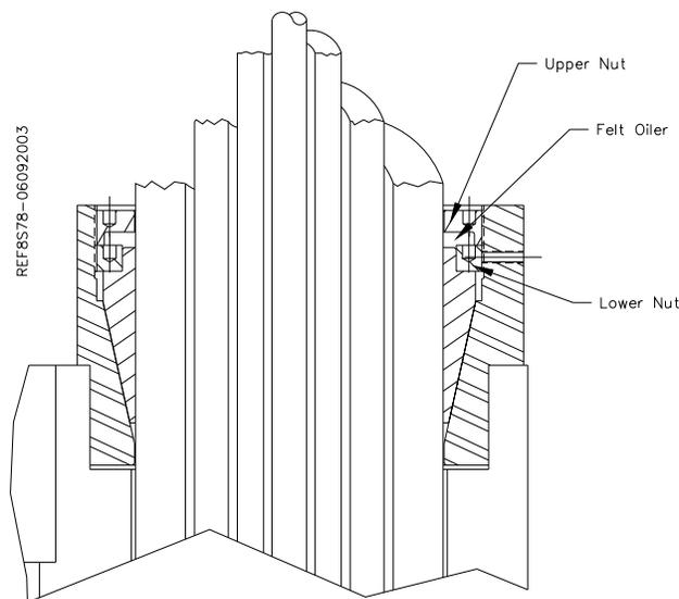
Slide the felt wiper back into place and tighten the Upper Nut back down.
