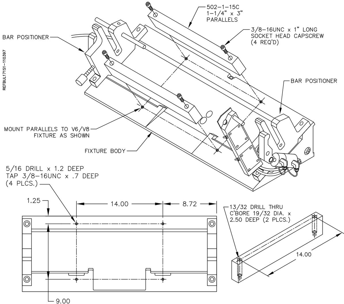
Some V-6 engine blocks (for example Buick V-6) have main bearing bores that are too low in respect to the pan rails. This presents a problem of the locator bar bottoming out in the bar positioners before the block is properly clamped. Positioning the 502-1-15C parallel set as shown below will raise the block enough to provide proper clamping.
