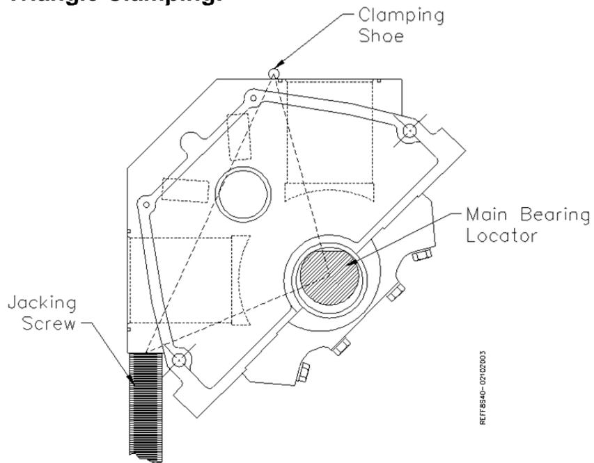
Adjust the height so the shoes rest on the clamp points. Tighten the clamp leg handles. Actuate the clamp shoes by turning their knobs. Apply pressure to the two clamps as evenly as possible to avoid tipping the block up on one side.
