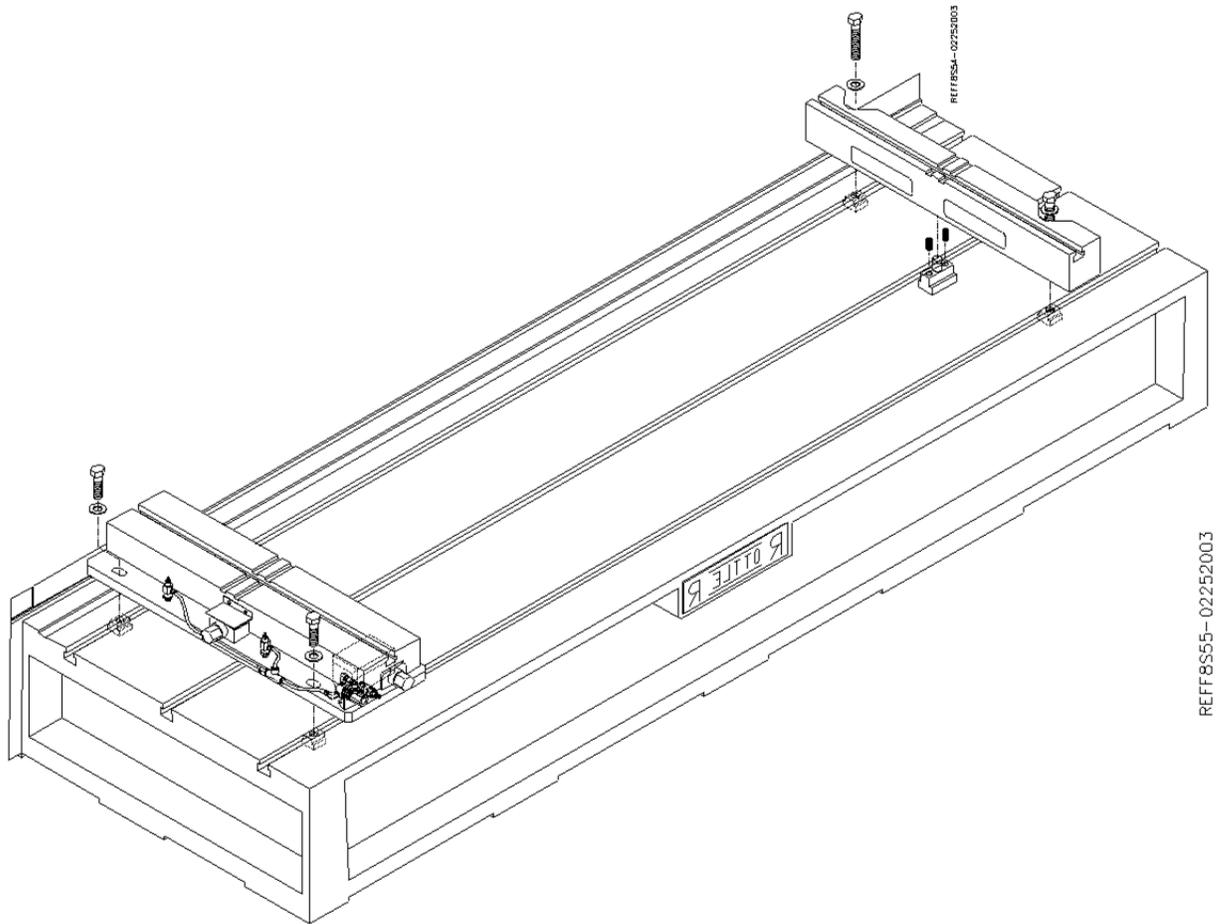
Select the set of V cradles for the block you are going to be machining. There are various types of cradles that can be used on this fixture. There are risers available also that can be mounted to the cradles to accommodate certain blocks. For cradle and riser selection refer to the Options section of this manual. The CAT 3500 series cradle is shown in this example.
