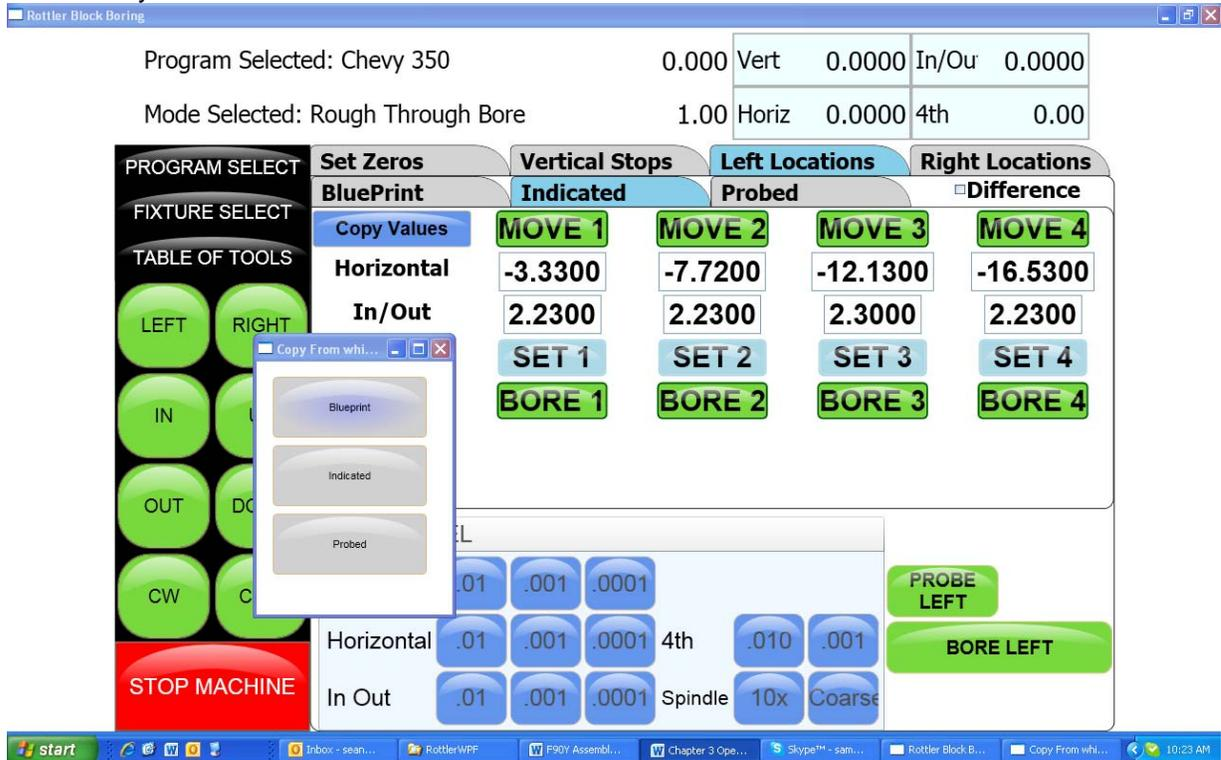
Press the Move 1 button. The machine will move to the first cylinder and stop at the centering position. Manually indicate the cylinder in using the Horizontal and In/Out handwheel. Once the cylinder is centered press the Set 1 button. This will transfer the current position of the machine into the first set of Data Boxes. Repeat this process for all the cylinders that need to be indicated.
