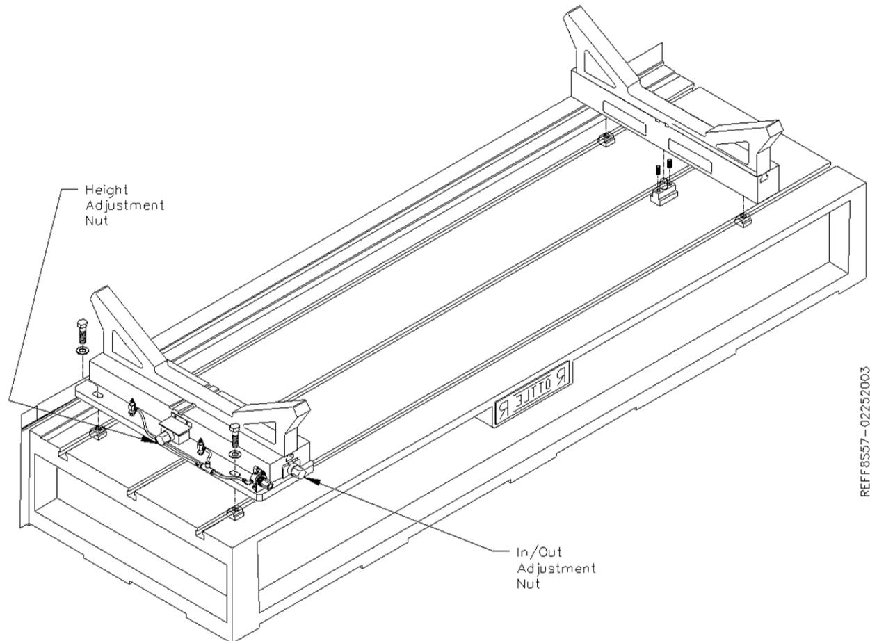
Lower the block slowly down into the cradles. Using a heavy soft mallet, tap the sides of the cradles to allow the block to settle into position. The block is now ready for alignment.
