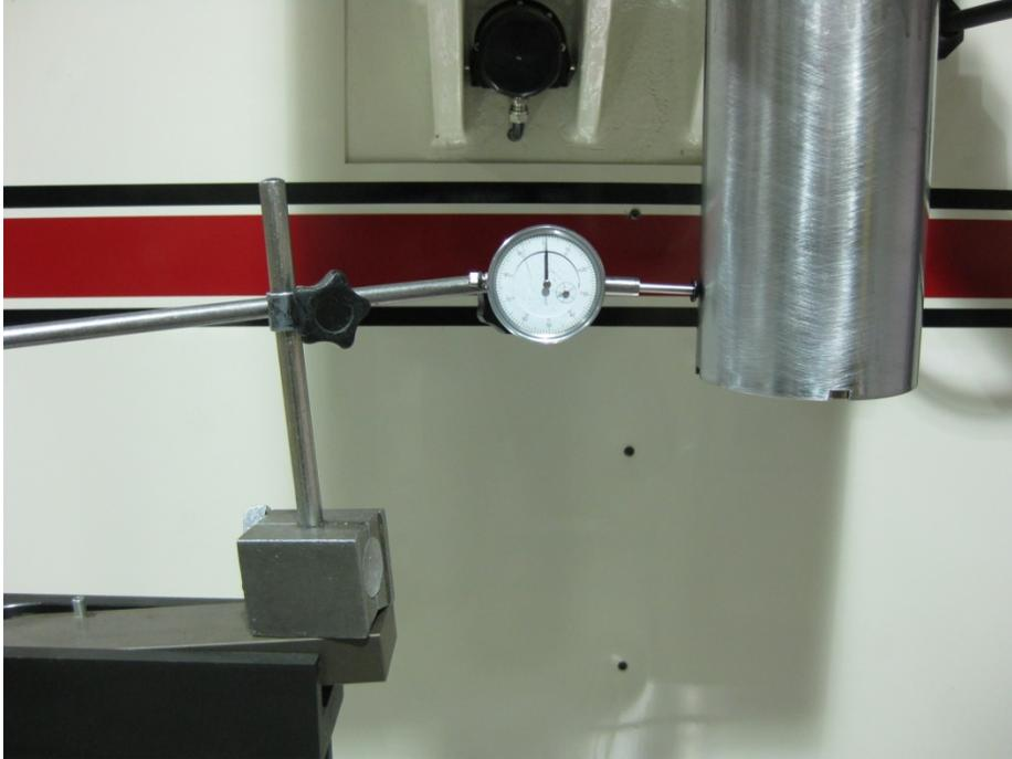
Bring the machine spindle in contact with the indicator.
