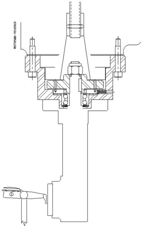
Put some pressure on the indicator. Using the In/Out handwheel move the indicator from one side to the other noting the amount of difference. Keep the indicator on that side of the head and rotate it half of the noted distance. Repeat this procedure until there is less than .0005" variance.
