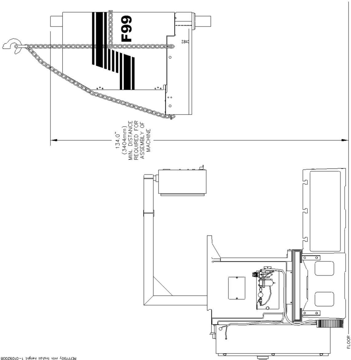
**F90Y Using Fork Lift & Angle Steel Brackets:**
