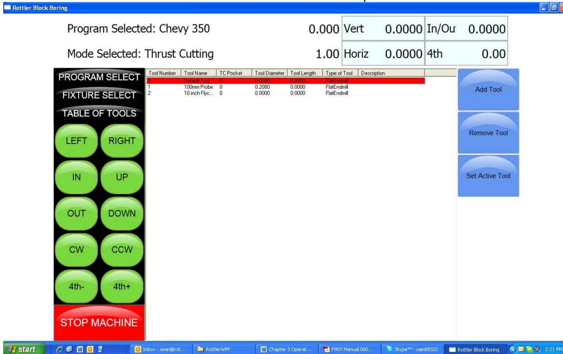
The 100mm Probe is Tool 1. The 10” Fly Cutter is Tool 2.
