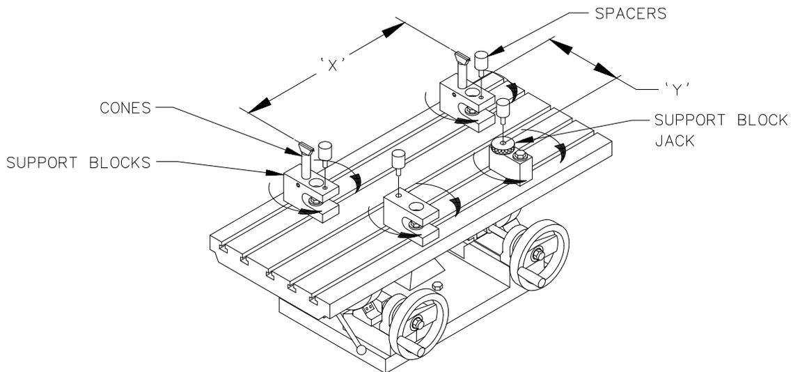
Place the head on the support blocks. Elevate the cones to 'hook' the two ports (bosses) on the head and tighten their set-screws. Adjust the position of the front support blocks if necessary. Tighten the hex bolts on the support blocks. Push the head back firmly into the cones. Adjust the support block jack to eliminate any rocking of the head. Do not tighten the head clamp handle assembly yet.
