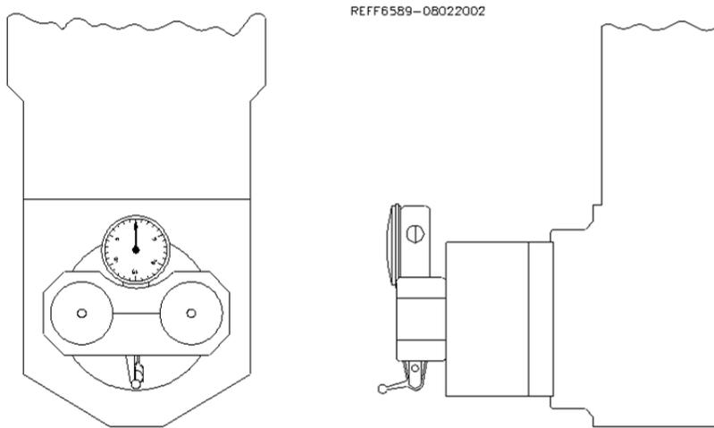
Using the Horizontal handwheel move the indicator inside the main bore, making sure the indicator is not touching the main bore at this point. You will be indicating both sides and the bottom of the saddle, generally the cap is not used to indicate from.
