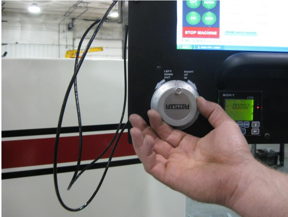
The movement shown on the indicator should be .001", plus or minus .0002". If not, an adjustment is needed.
