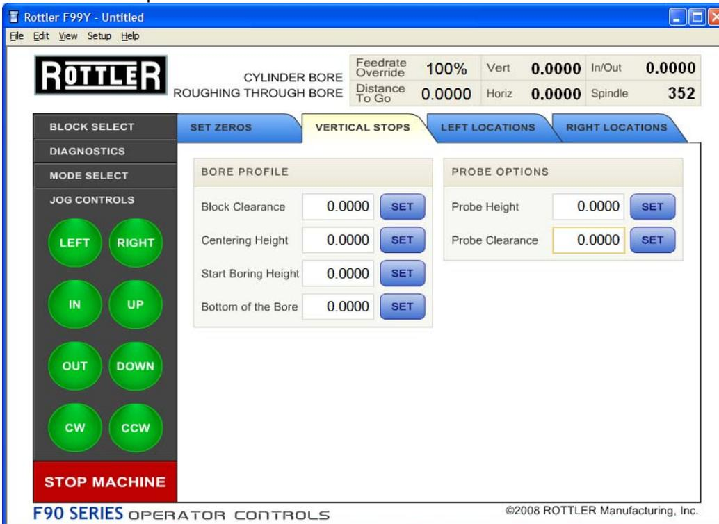
Move the machine spindle away from the dial indicator a few inches, and press "Move to Zeros".
