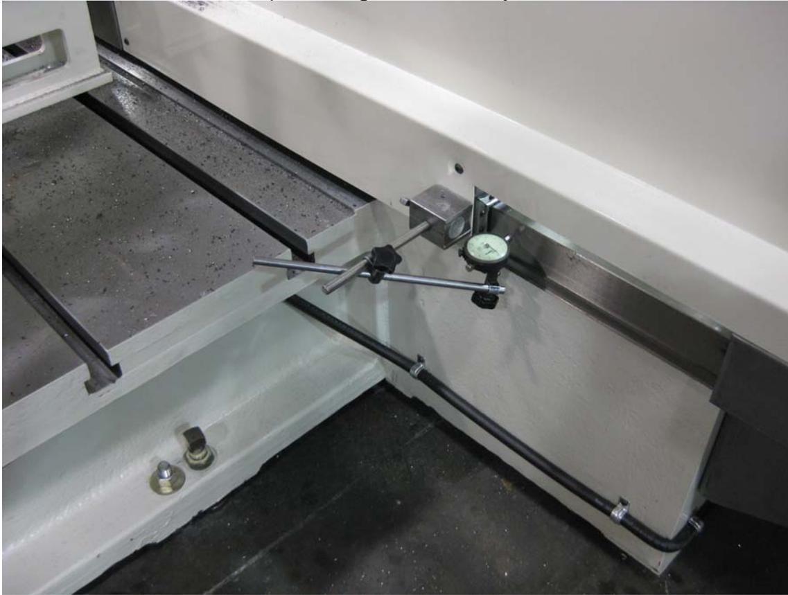
Now using the handwheel in .010" per click mode, move the column back and forth, about two turns on the handwheel in each direction at a rapid rate.
