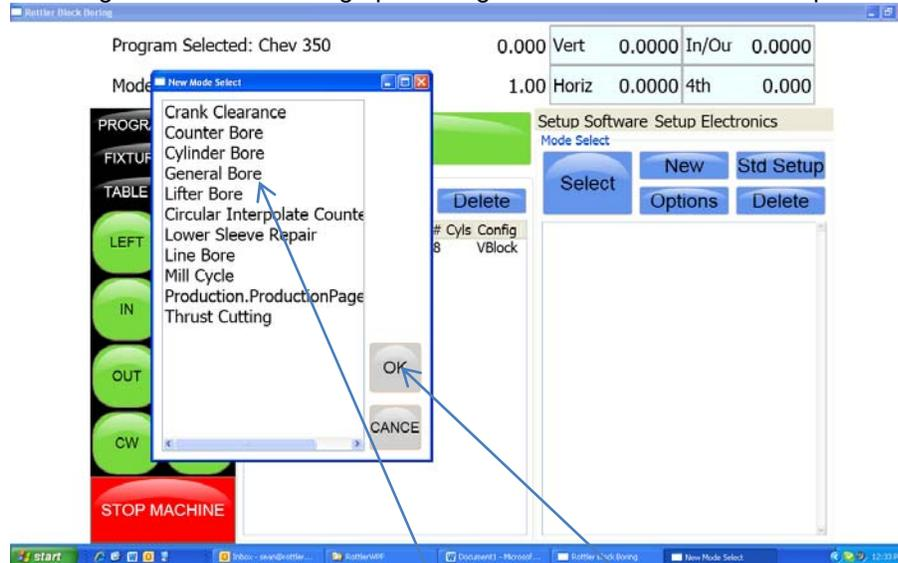
Select the operation you want to create and then press OK. This will place a general Bore operation under the Cylinder bore mode in the right hand section.
