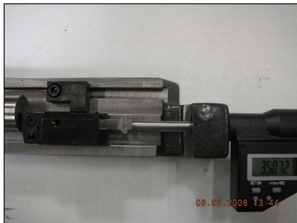
The micrometer is now set up for use with this cutter head.
