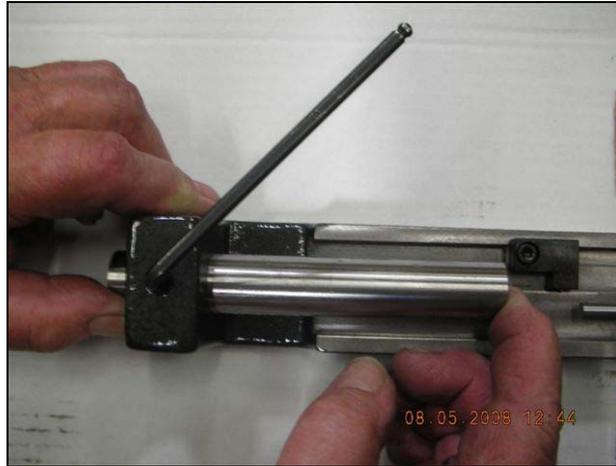
Place the tool holder used to bore the hole into the micrometer frame. Slide the location nub on the back of the tool holder gently up against the end of the digital micrometer shaft.
