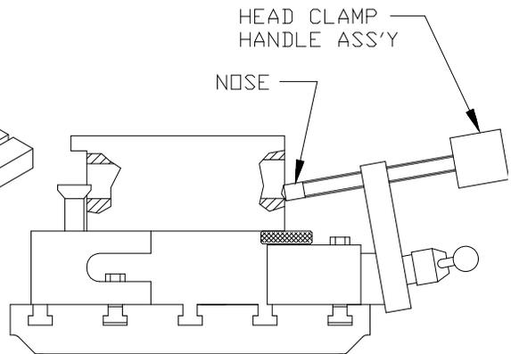
Visually check for clearance between the cutterhead and head fixture tooling pieces, especially the head clamp handle, assembly. The head should be approximately centered in the path of the cutterhead.
