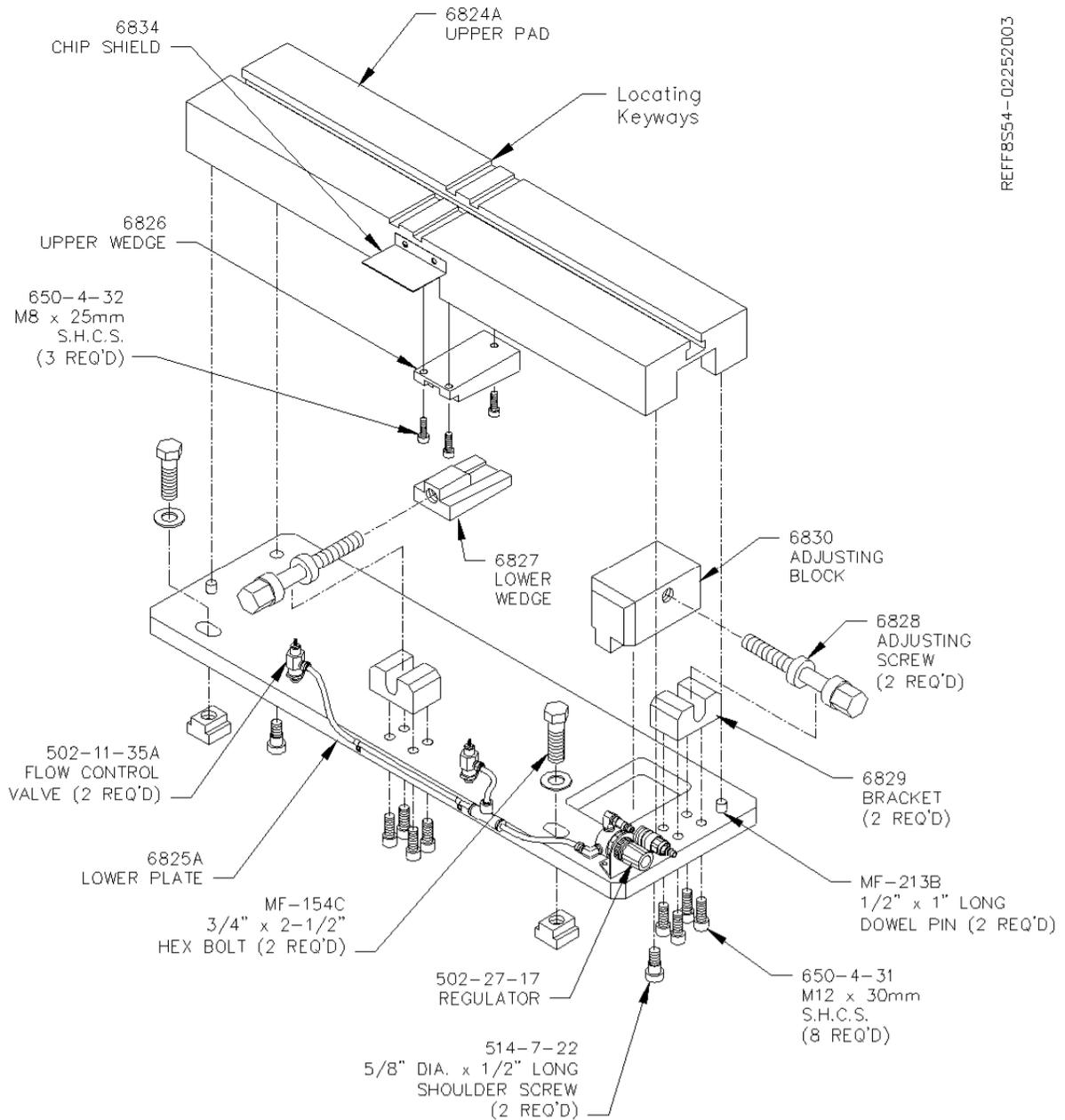
Once both parallels are installed on the machine bed, place a magnetic indicator on the spindle towards the main bed. Indicate the adjustable parallel into the stationary parallel to within .002" on the In/Out and height. This lines the fixture up close so the block can be loaded and then use minor adjustments on the fixture to line the block up.
