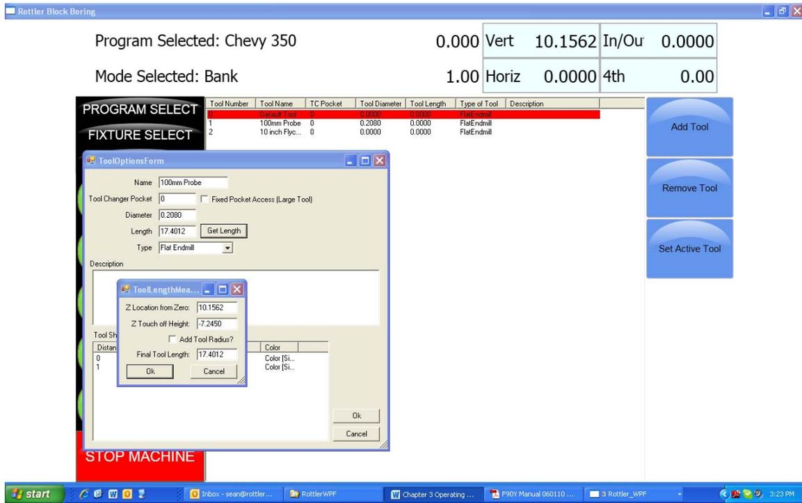
Select OK on both windows. This will put the Total tool length into the Table of Tools.
