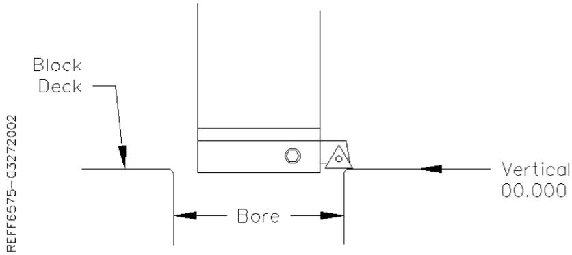
The zeros points for all axis have now been set. All the numbers entered from this point on will reference these zero positions. You are finished with the Set Zeros screen, select the next Tab to the Right, Vertical Stops.
