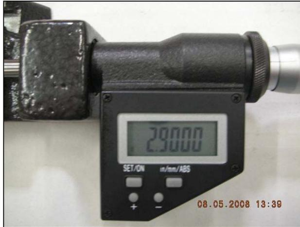
Determine which cutter head bore range the micrometer is going to be used on. ( example; 2.9 – 6.0 )
