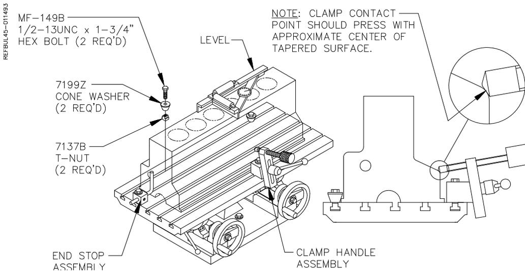
Check that all bolts and holdowns are tight. Loosen table clamp and level head surface of block in both directions. Lock table clamp and recheck block for level.
