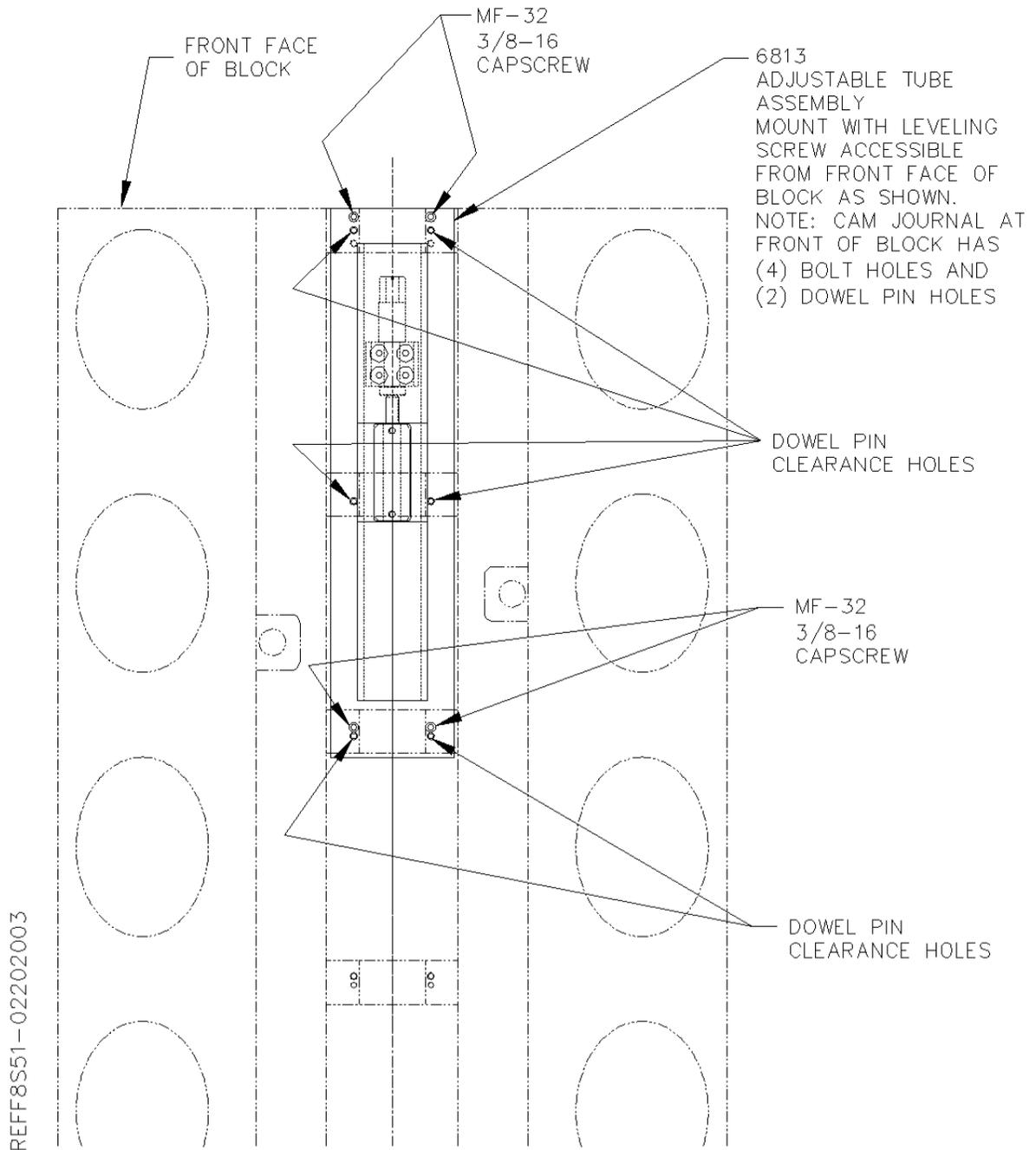
The upper and lower leveling pads, bracket and screw are already installed in the adjustable tube.
