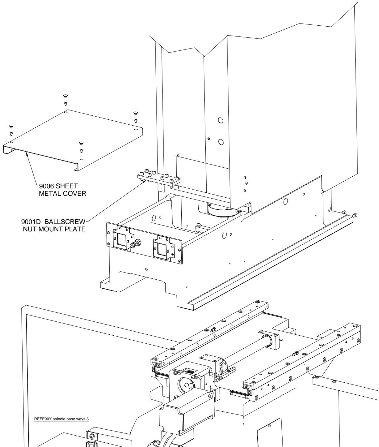
**Spindle Base Assembly with Column cont.:**
