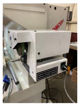
Step 5: Wire the sharpener by running the power cable through the side of the cabinet and over to the breaker in the electrical cabinet. The sharpener is wired by attaching the red and black power leads to the T1 and T2 terminals on the lower part of the breaker as shown in the figure below. The green and yellow ground cable can be connected to any open ground terminal in the terminal block behind the breaker.
