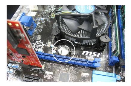
Push the battery retention clip away from the battery. When the clip is released the battery will pop up.
