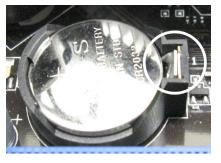
Remove the battery and place new battery in the battery holder.
