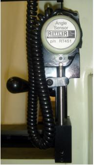
Example: level reads 0.04 to the left, when rotated 180 degrees to the right it should read minus 0.04.
