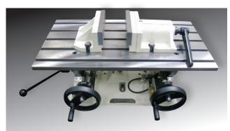
Two piece vice allows parts like exhaust manifold and main line bearing caps to be clamped, then leveled and surfaced.
