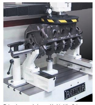
Extra clearance below and behind the fixture allow high deck height V-Blocks to be rolled to both banks for surfacing without removing the block from the machine.
