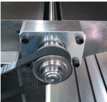
Belt drive precision ball screw for Turcite coated workhead.
