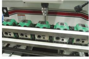
**Universal Chuck** Universal Chuck can be used for odd jobs like drilling out broken bolts and tapping threads
