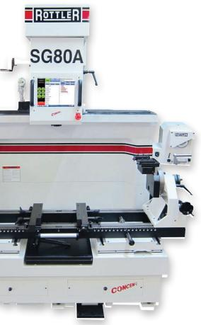
The massive envelope and the optional Tilt Fixture allows very large heads to be set up and leveled, and clamped with the roll fixture or tower clamps.
