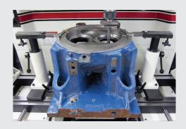
**Tower Clamps** Adjustable tower clamps allow quick clamping of odd jobs.
