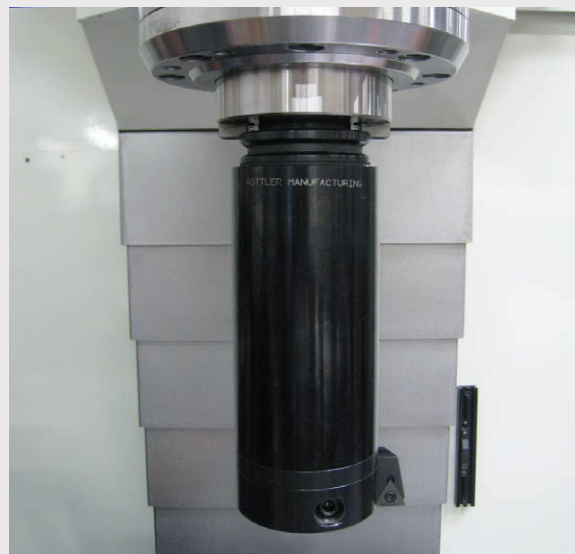
Rottler Boring and Sleeving Cutterhead installed in massive heavy duty F69ATC Spindle.
